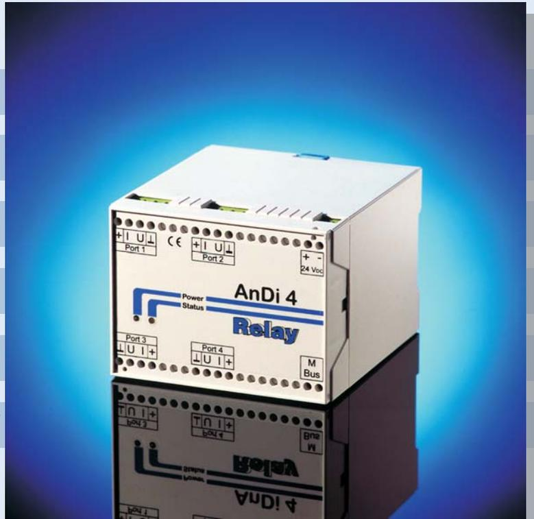
The AnDi 4 allows capturing of analog measured data such as pressure, temperature or speed by a M-Bus installation. The connection of standard industrial sensors with 0/4...20 mA or 0...10V signals is possible.
